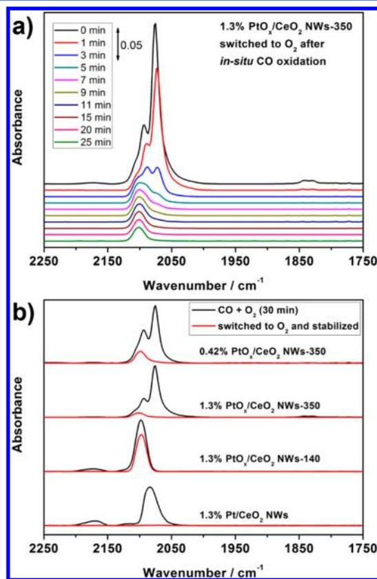
Figure 4. In situ IR spectra of PtO<sub>x</sub>/CeO<sub>2</sub> NWs under CO oxidation conditions: (a) reaction of adsorbed CO intermediates with O<sub>2</sub> over a sample of 1.3% PtO<sub>x</sub>/CeO<sub>2</sub> NWs-350 after stabilization under the CO oxidation conditions; (b) stabilized peaks under CO oxidation conditions and the residual peaks after O<sub>2</sub> treatment for the PtO<sub>x</sub>/CeO<sub>2</sub> NWs samples.
