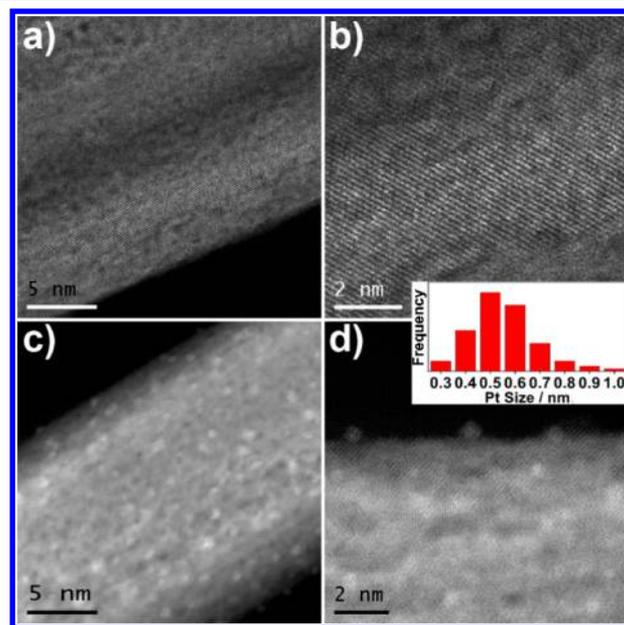
**Figure 1.** Aberration-corrected STEM images of 1.3% PtO<sub>x</sub>/CeO<sub>2</sub> NWs-140 (a, b) and 1.3% PtO<sub>x</sub>/CeO<sub>2</sub> NWs-350 (c, d). The insert in panel d shows the size distribution of PtO<sub>x</sub> clusters on the sample of 1.3% PtO<sub>x</sub>/CeO<sub>2</sub> NWs-350 obtained from measurements of the size of over 150 nanoclusters.
