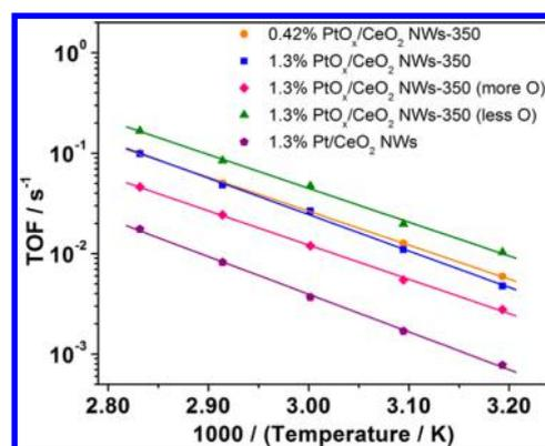
Figure 2. Catalytic activity on CO oxidation over PtO<sub>x</sub>/CeO<sub>2</sub> NWs. Error bounds are estimated to be about ±20%. The TOF value of 1.3% PtO<sub>x</sub>/CeO<sub>2</sub> NWs-140 was less than 10<sup>−4</sup> s<sup>−1</sup> at 50 °C. The TOF value of the pure support CeO<sub>2</sub> NWs was 4.1 × 10<sup>−5</sup> s<sup>−1</sup> at 200 °C.
