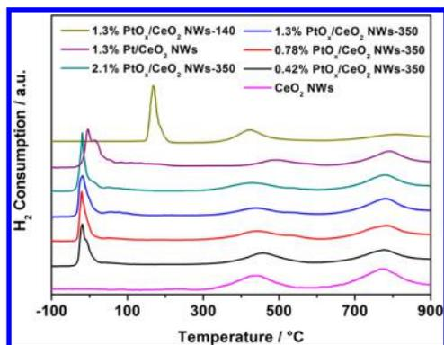
Figure 3. H<sub>2</sub>-TPR profiles of PtO<sub>x</sub>/CeO<sub>2</sub> NWs samples.
