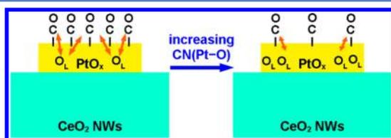
**Figure 7.** Proposed effects of the increasing CN(Pt–O) on the low-temperature catalytic CO oxidation over subnano PtO<sub>x</sub>/CeO<sub>2</sub> NWs. O<sub>L</sub> represents the active lattice oxygen of PtO<sub>x</sub>, Pt–O–Ce linkages, and/or some oxygen species very close to Pt atoms.
